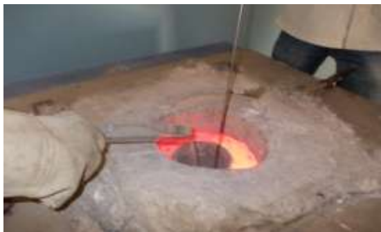
Fig. 1: Pouring and stirring of reinforcement in stir casting method
